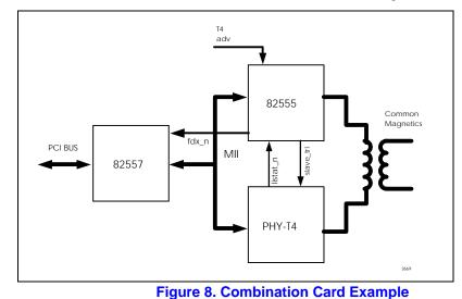
The figure below illustrates an 82557/82555/PHY-T4 solution in a block diagram.
